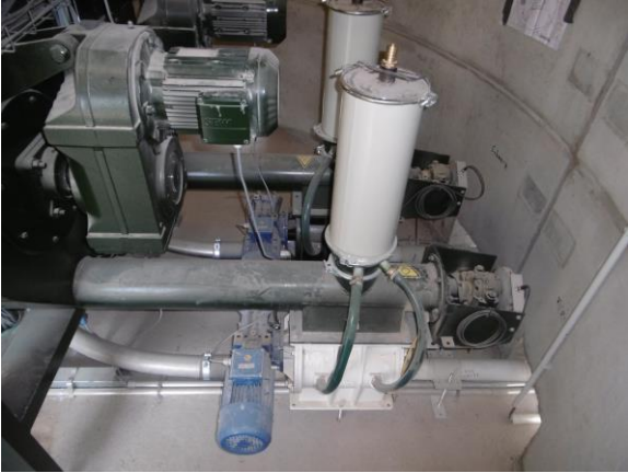
2 separate Dosing lines: To burner "white" line To burner "black" line
